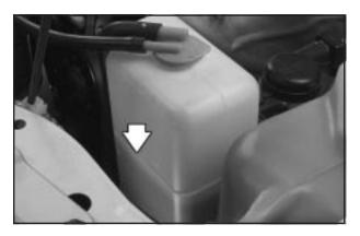
The coolant level should be at or above FULL. If it isn't, you may have a leak at the pressure cap or in the radiator hoses, heater hoses, radiator, water pump or somewhere else in the cooling system.
